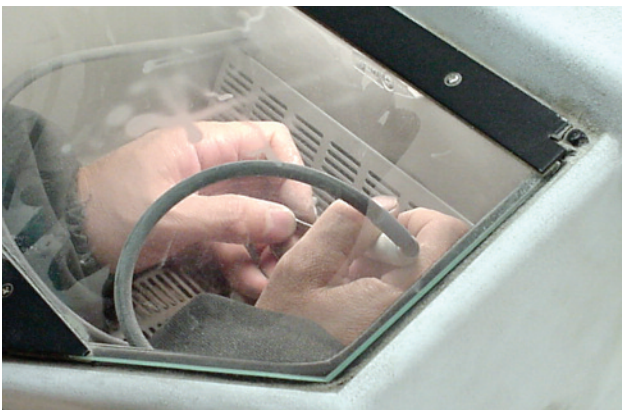
Figure 22. Micro-etch the inside of the bands using abrasive blast.
