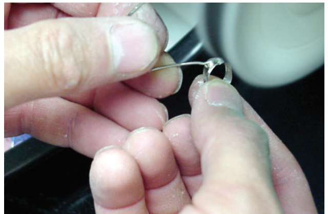
Figure 21. High shine the solder joint as well as the .045 wire. Do not touch the Teflon roller or it will mark and be damaged.
