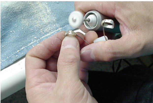
Figure 20. Using a heatless stone, smooth out the solder joint at the molar band.
